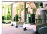
Chaole Series Vertical Pulverizer Capacity: 1.2 - 3.5 MTPH Power: 90 - 132 KW
