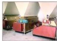
MUSL Series Crumbler Capacity: 6.0 - 25 MTPH Power: 7.5 - 22 KW
