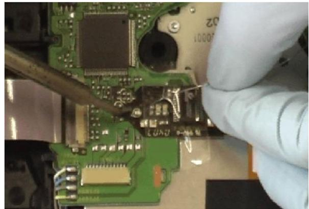
Figure 4.1: Example of installing a modification chip to bypass region locking
